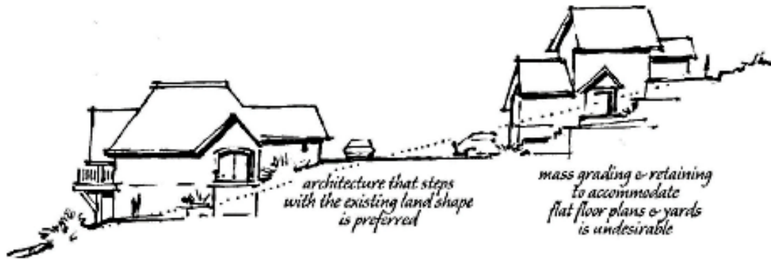
Figure 4-22. Hillside Adaptive Architecture
